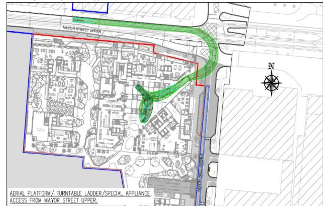
Figure 6.2: Extract of Dwg. No. R064-210, 'Autotrack – Ground Level – Fire Tender', Rev. E. Source: CS Consulting, January 2021. Cropped by TPA, January 2021.
